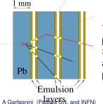
Target: Pb + nuclear emulsion bricks alternated to plastic scintillator strips Spectrometer: drift tubes for momentum measurement and magnet inner walls instrumented with 22 RPC planes for muon charge identification
